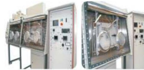
Glove box with the deposition system for nano technology applications
