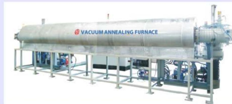
continuous heating under vacuum and continuous cooling under natural/inert gas environment. A vacuum pumping system provided on either side of the collar to achieve a ultimate vacuum of  $1 \times 10^{-6}$  m.bar. It has an internal diameter of 300mm ID x 550mm cylindrical length and a copper coil is brazed on the collar for water circulation for effective cooling. A gas inlet system also
