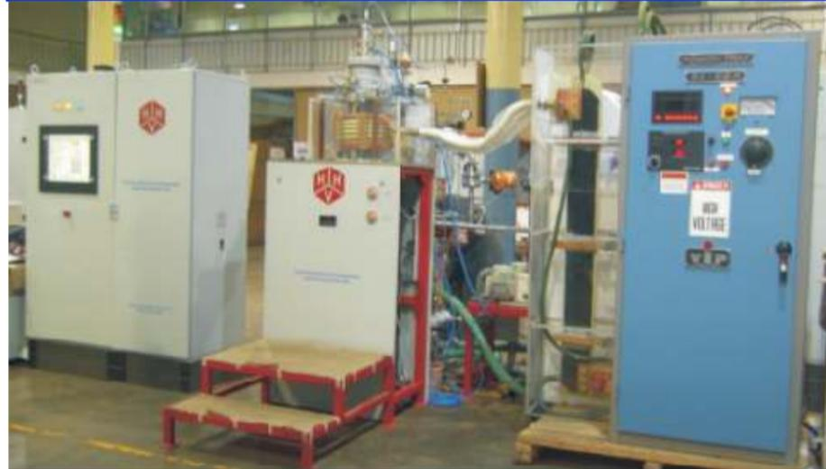
This laboratory furnace is a versatile facility designed to develop various crystals and work with a variety of doping materials.
