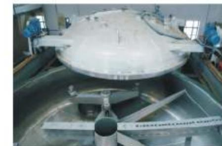
Top dished end moving mechanism
