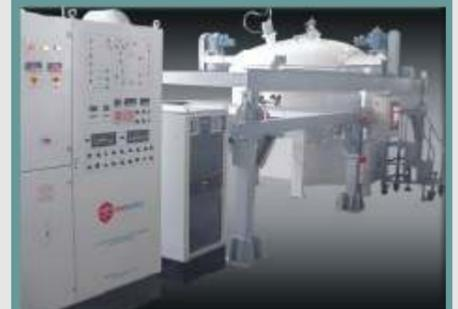
A telescope mirror coater at Girawali to coat the concave, 2.2 metre dia. mirror has a thickness of 200mm & weighs about 2.50 tone
