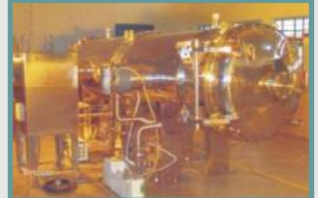
High vacuum system to find the best focal plane of an integrated UV telescope and to fix the right focal plane with a detector, in a laboratory-created space environment
