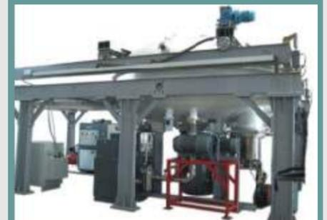
HHV telescope mirror coater at Devasthal to coat 3.7 diameter metres mirror, a thin cross section only 12 cm thick and a large weight 4.5 tonnes
