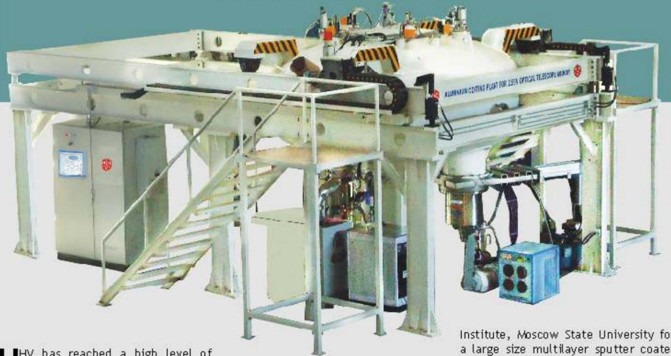
HHV has reached a high level of expertise in engineering, manufacturing and commissioning of very complex and highly precise coaters for large size, heavy weight and thin telescope mirrors
