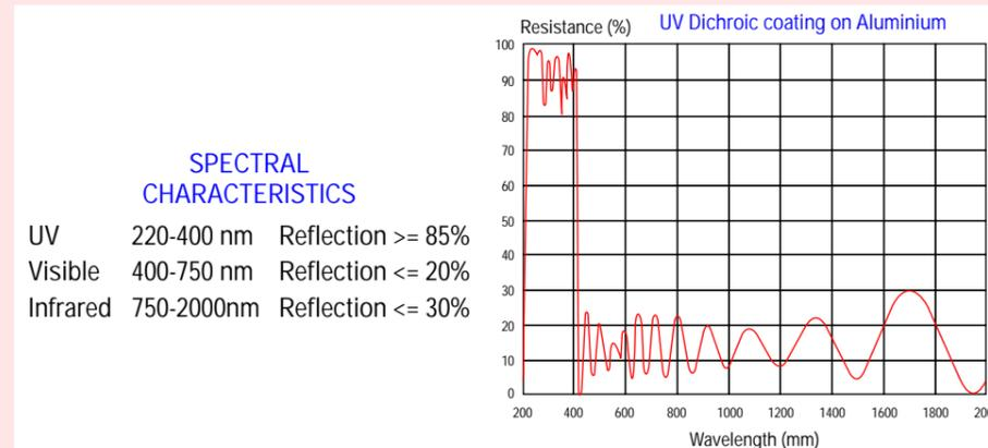
UV Reflector coating on Aluminium Extrusions and its spectral characteristics
