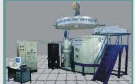
First telescope mirror coater at the Hanle observatory to coat the 2.1 metre diameter telescopic mirror of 1 tonne weight
